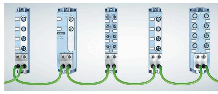
ET 200AL in IP65/67– by means of an ET 200AL PROFIBUS/PROFINET interface module, the ET 200AL I/O modules are combined in two rows to form one station.
